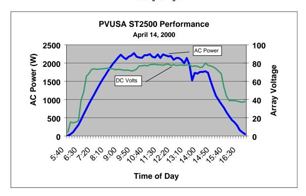
The following inverter efficiency data illustrates the high efficiency over a wide range of power levels. The ST2500 achieves an overall inverter efficiency of 90% or greater above 500 watts in the laboratory. The 6 minute interval data below illustrates real-world efficiencies over the power range during 35 to 45°C ambient temperatures and varying sunlight.
